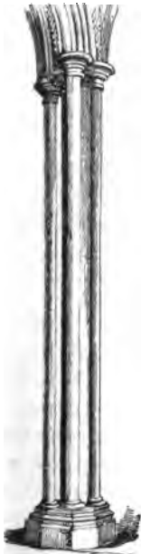
88. Salisbury Cathedral, A.D. 1220—1237. Clustered pillar with detached shafts.
